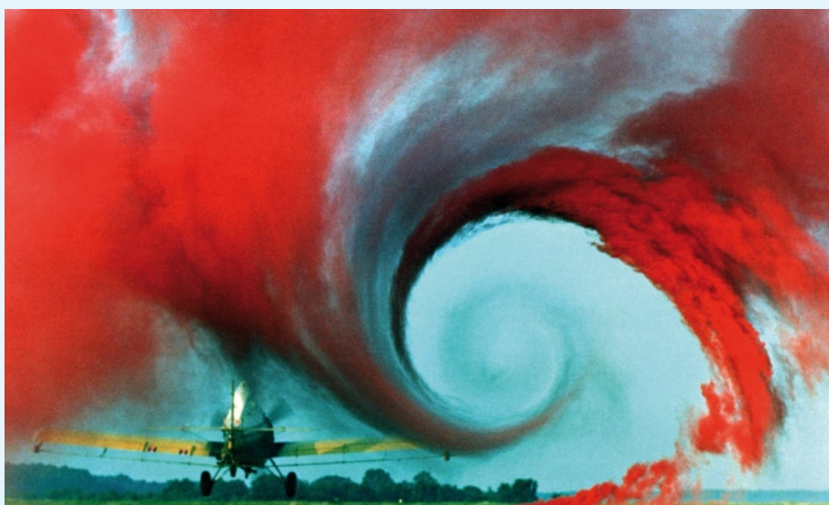
A NASA photo showing a wake vortex illuminated by a smoke-generating flare.
